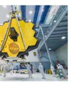
The best way to make a really powerful telescope is to build a big mirror. The James Webb Space Telescope has the largest mirror of its kind that NASA has ever built—so big that it can't fit inside a rocket without folding up. Together, the 18 hexagonal mirror segments span 21.3 feet.
